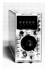
The TEKTRONIX 5B31 Digitally Delayed Time Base, a new plugin in the 5400-Series Oscilloscope line, brings new measurement accuracy and operating convenience to many delaying sweep applications. The delay system — a crystal-controlled clock, a digital counterlinates one-count ambiguity in the counter — replaces the usual delaying sweep.
